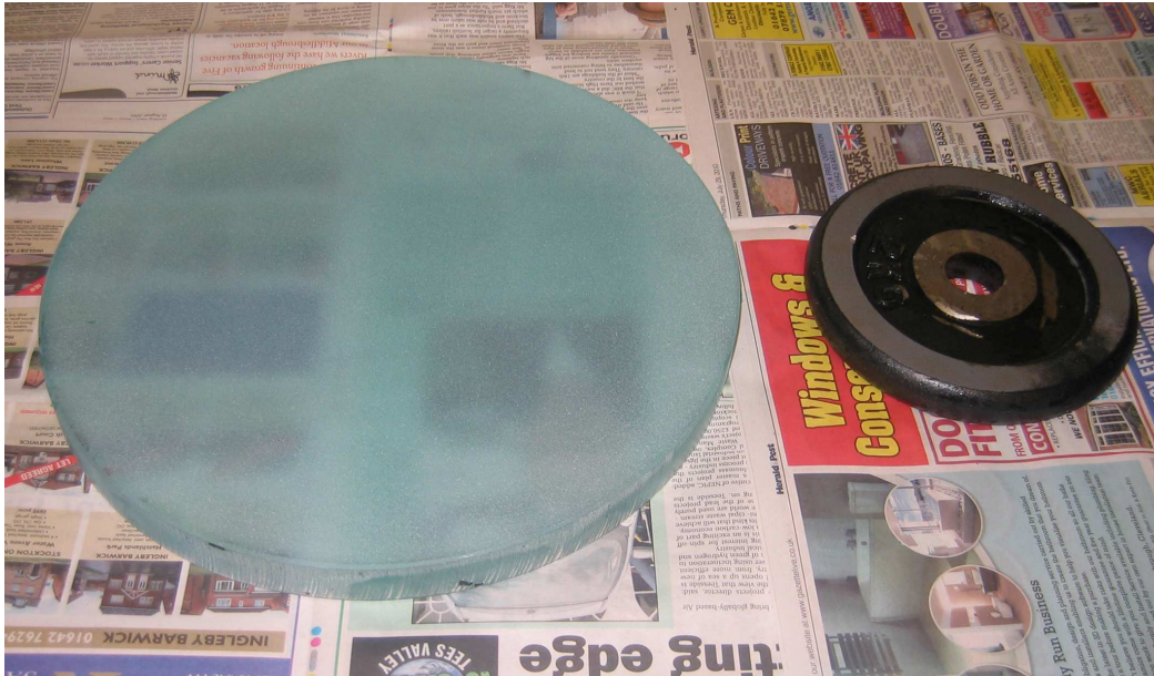
The mirror and grinding tool after 2 hours work.
