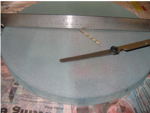
Measuring the sagitta with feeler gauges or a twist drill.
